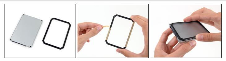
• For 7 mm SSDs, you'll need to apply a spacer to ensure a good fit.
